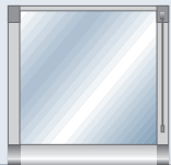
mounting on casement with cord drive and SunTape lateral guiding from bottom to top
