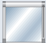
mounting on casement with SunTape lateral guiding
