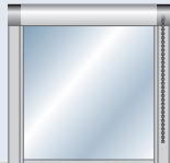
wall or ceiling mounting with clip support, side pull drive, side guiding
