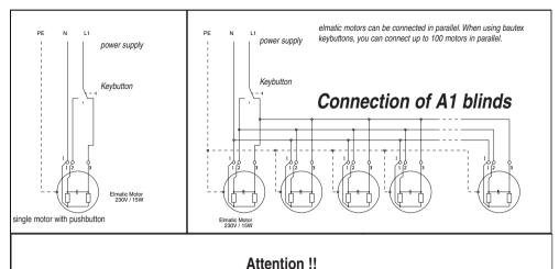
Elmatic motors do not have limit switches. Therefore you may only use key buttons. Remote controls may not admit operation by locking switch.
