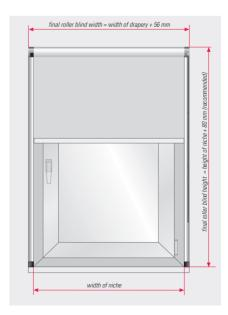
side pull drive or electric drive with SunTape side quiding wall mounting
